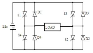
Fig 3Thyristor as an inverter
