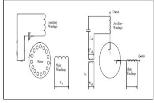
Fig9. Split phase induction motor modeling
