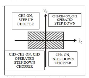
Fig. 8 Working of Four Quadrant Chopper
