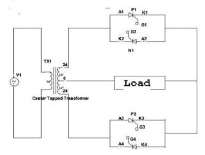
Fig.5 Single Phase Cycloconverter
