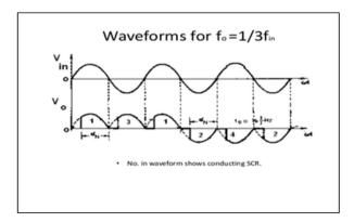
Fig. 6 Working of cycloconverter for each cycle.
