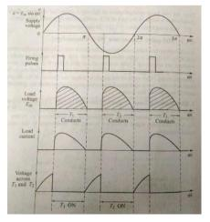
Fig.2 Output Waveform for Rectifier
