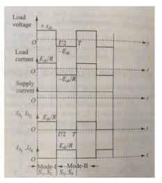
Fig.4 Voltage and Current waveform for inverter
